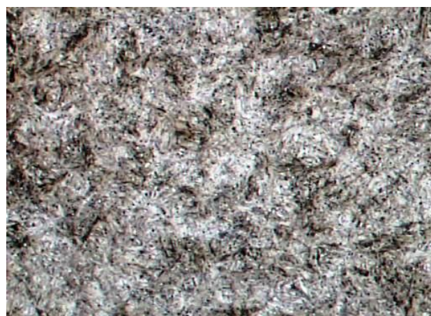
micrography x500 ferrite free heat treated structure with undissolved carbides
