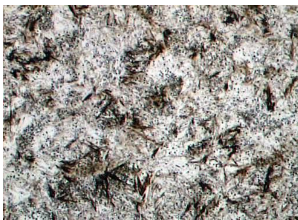
micrography x500 martensite with undissolved carbides mikroskopische world of iron and steel
