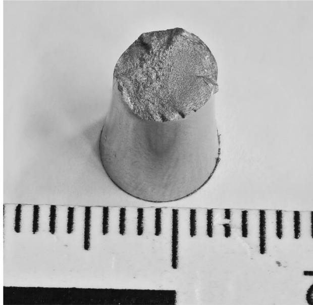
*Figure 145 - Fracture surface of specimen F1B (S355J2)*
