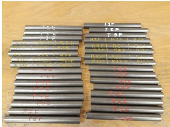
Figure 45 - Raw specimens obtained for the material 11SMnPb30 and 11SMnPb37
