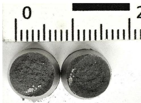
Figure 89 - Fracture surfaces 11SMnPb37
