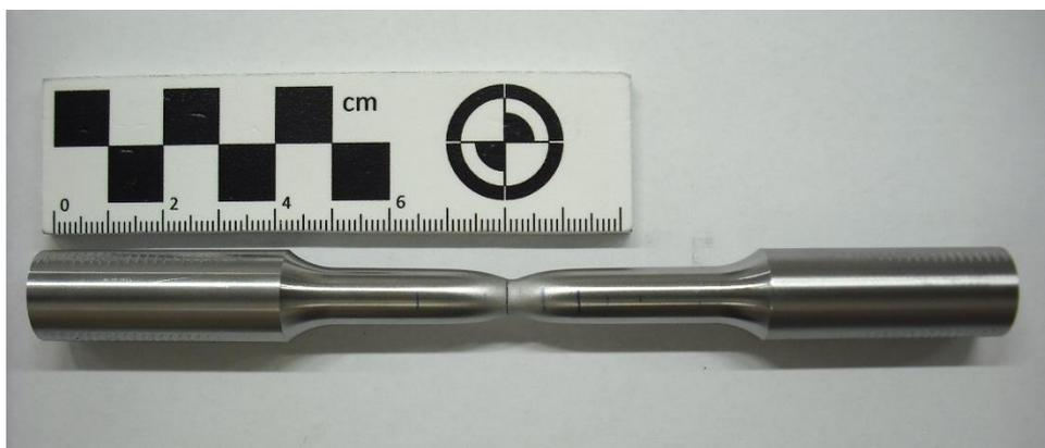
Figure 56 - Specimen of S235JR after the tensile test
