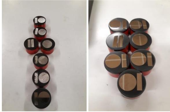
*Figure 4 - Metallographic specimens before (left) and after (right) polishing*
