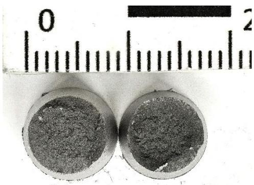
Figure 88 - Fracture surfaces 11SMnPb30
