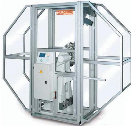
Figure 105 - Charpy's pendulum
