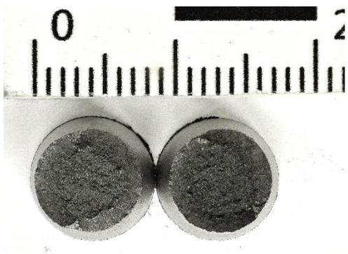
Figure 86 - Fracture surfaces 11SMn30
