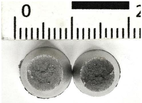
Figure 84 - Fracture surfaces S235JR
