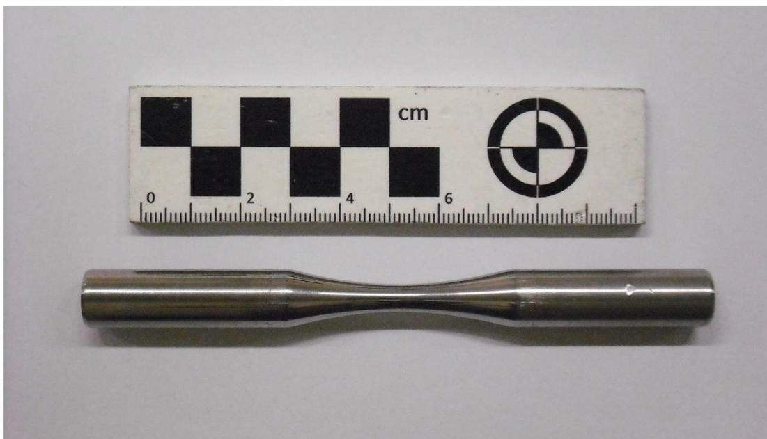
Figure 52 - Rotating bending fatigue test's specimen
