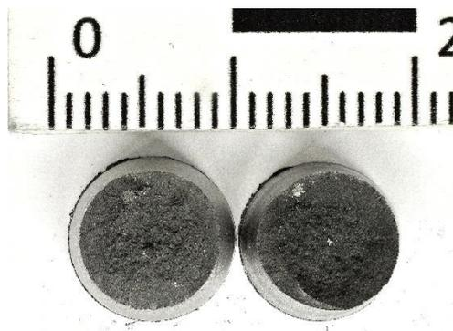
Figure 87 - Fracture surfaces 11SMn37
