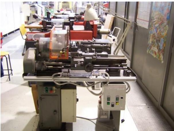
*Figure 137 - Lathe used for polishing operations*
