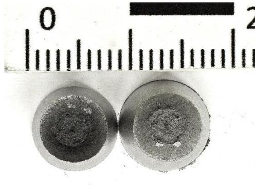
Figure 85 - Fracture surfaces S355J2
