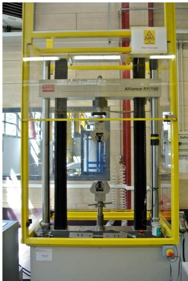
Figure 53 - Tensile test machine
