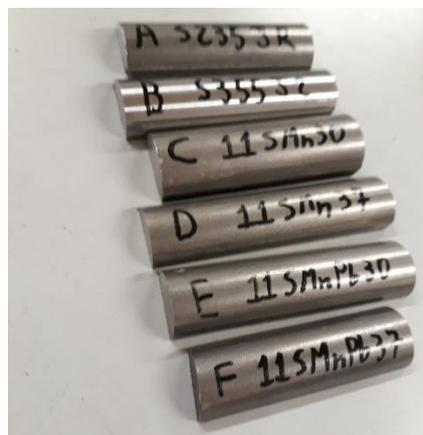
Figure 46 - Samples for chemical analysis
