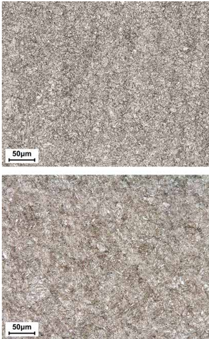
Figure 13.2 – Metallographic appearance of the tempered martensitic structure of steel grades EN 42CrMo4 (top) and EN 36CrNiMo4 (bottom) [Exova S.r.l. Laboratories - Crema, Italy].
