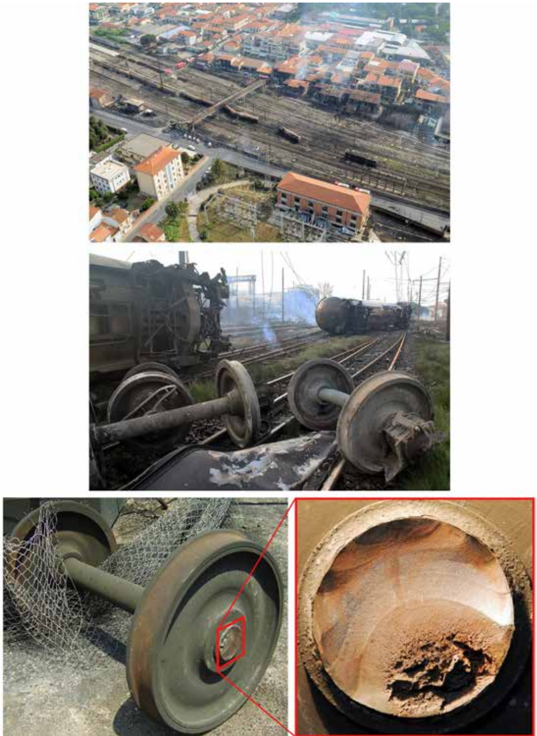
Figure 6.2 – Viareggio railway accident involving the freight train 50325 Trecate-Gricignano. Detail of the fracture surface of the axle broken due to fatigue [pictures by POLFER, Viareggio railway accident, 29 June 2009].
