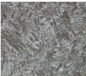
Hot-rolled Quenched and tempered Martensite and traces of bainite X500
