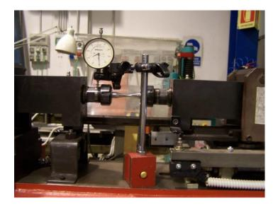
Figure 141 - Comparator applied to the spindle
