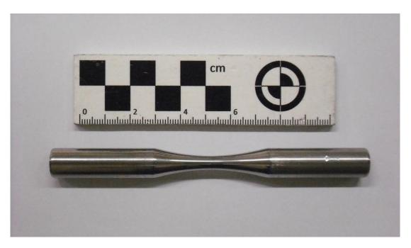
Figure 52 - Rotating bending fatigue test's specimen
