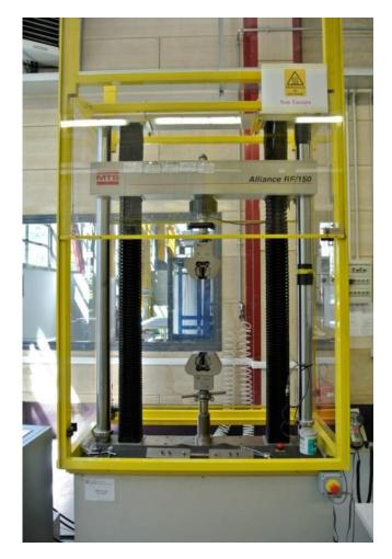
Figure 53 - Tensile test machine
