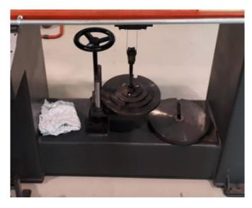
Figure 142 - Load applied to the machine
