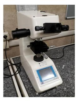
Figure 154 - Durometer for Vickers hardness tests
