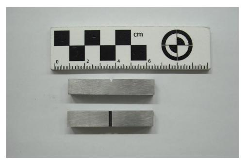
Figure 50 - Toughness test's specimens
