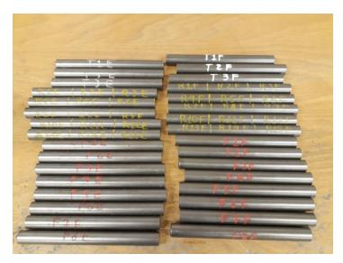
Figure 45 - Raw specimens obtained for the material 11SMnPb30 and 11SMnPb37
