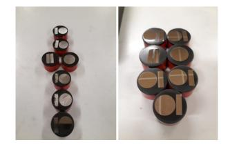
Figure 4 - Metallographic specimens before (left) and after (right) polishing
