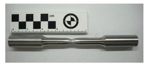
Figure 56 - Specimen of S235JR after the tensile test
