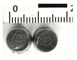
Figure 89 - Fracture surfaces 11SMnPb37
