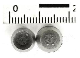
Figure 85 - Fracture surfaces S355J2
