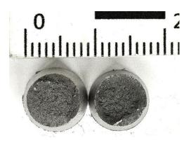
Figure 88 - Fracture surfaces 11SMnPb30
