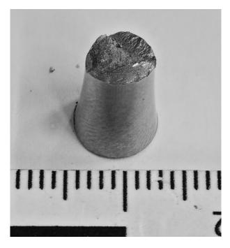
Figure 146 - Fracture surface of specimen F7E (11SMnPb37)
