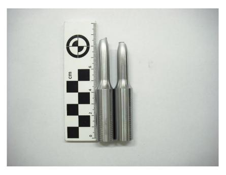
Figure 83 - Specimen after the tensile test
