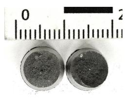
Figure 87 - Fracture surfaces 11SMn37
