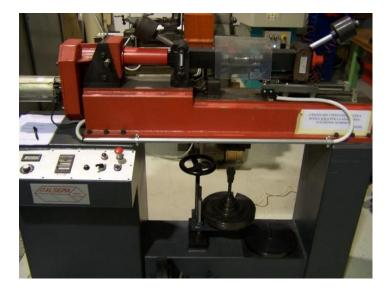
*Figure 139 - Machine for the rotating bending fatigue test*
