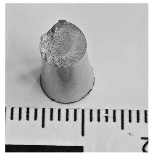
Figure 144 - Fracture surface of specimen F6B (S355J2)
