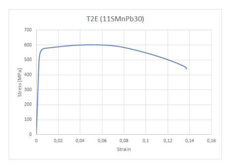
Figure 70 - Stress-strain curve specimen T2E (11SMnPB30)
